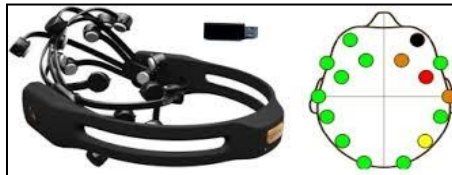
Figure 4: EMOTIV Epoch+ and 16 electrodes used on the scalp
