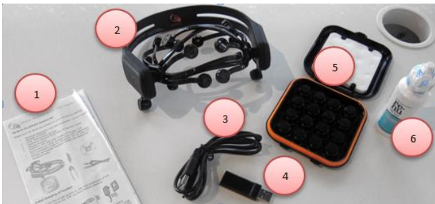
Figure 3: (1) Manual user, (2) Emotiv EPOC+, (3) USB charger, (4) USB wireless, (5) 16 Electrodes and (6) Saline solution
