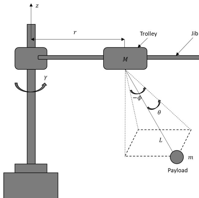
Figure 1. Tower crane system
