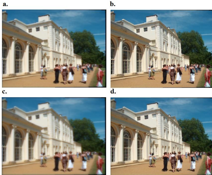
Figure 3. Image simulation of a. aberrated model at 555 nm. b. Al-doped CL at 555 nm. c. aberrated model at (470-650 nm). d. Al-doped CL at (470-650 nm).
