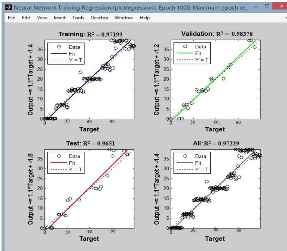
Figure 8. Regression plots of the artificial neural networks model
