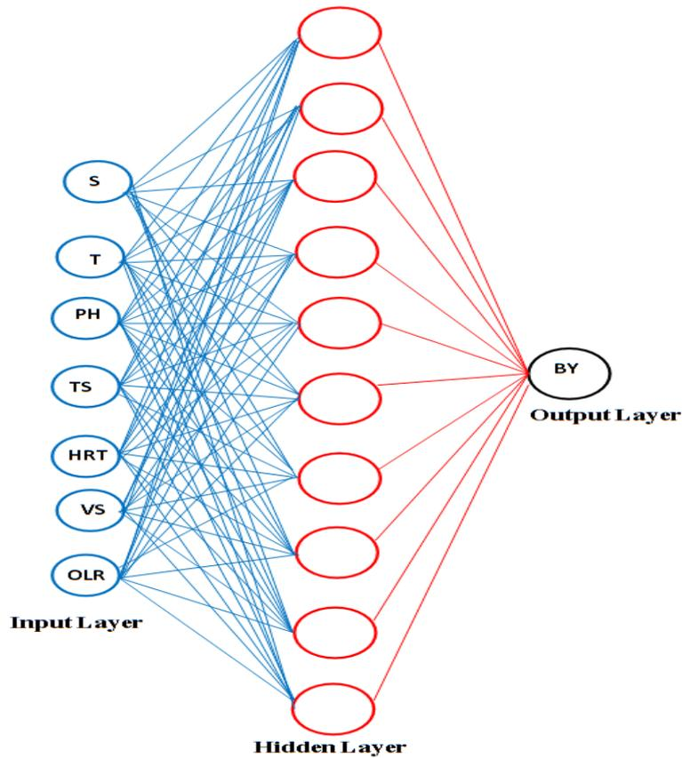
Figure 4. Artificial neural networks architecture
