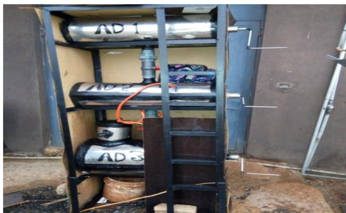
Figure 3. Three-stage continuous anaerobic digestion plant
