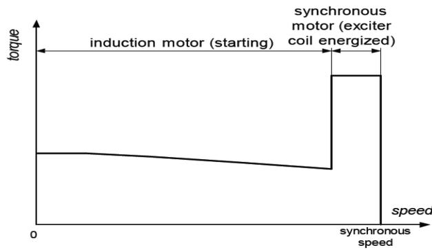
Figure 2. Torque vs. speed characteristic of a written-pole motor
