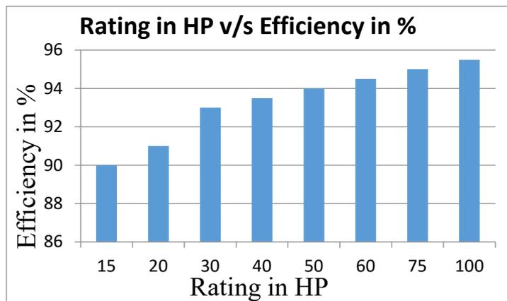
Figure 4. Rating in HP vs. efficiency in % for 4-pole, 240 Volt single-phase written-pole motor
