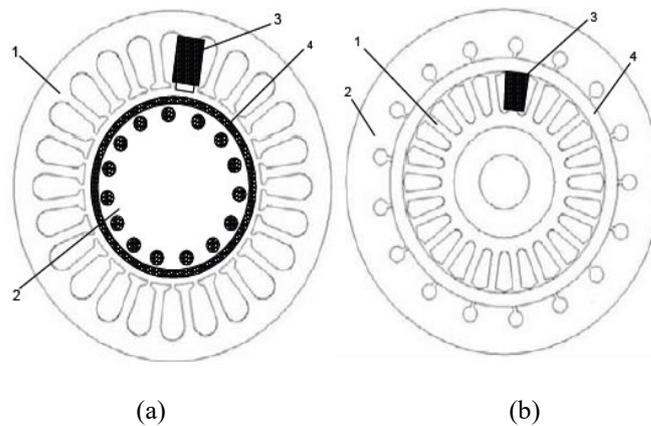
Figure 1. Construction of a written-pole machine: (a) with inner rotor (b) with outer rotor.
