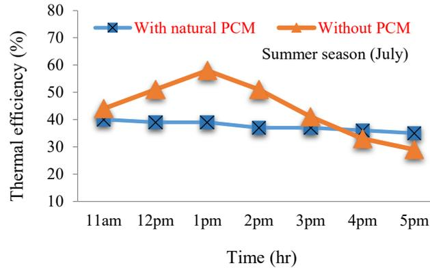
Figure 6. Variation of thermal efficiency with PCM and without PCM condition in July
