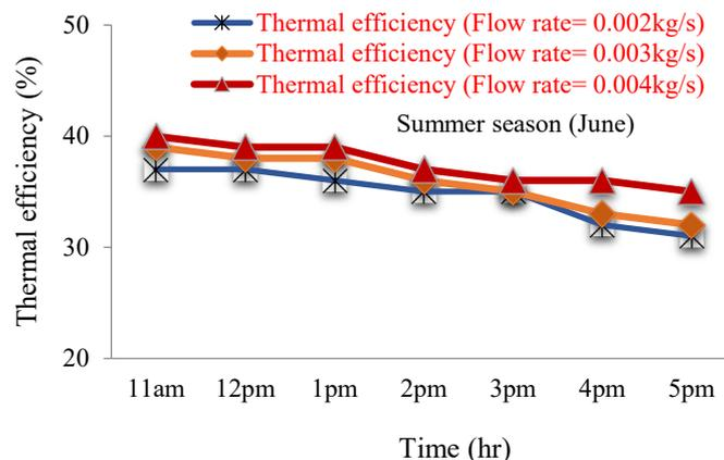
Figure 5. Variation of thermal efficiency at different water-flow rates at different times
