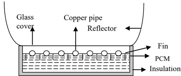
Figure 1. The sectional views of a CPC solar collector with PCM
