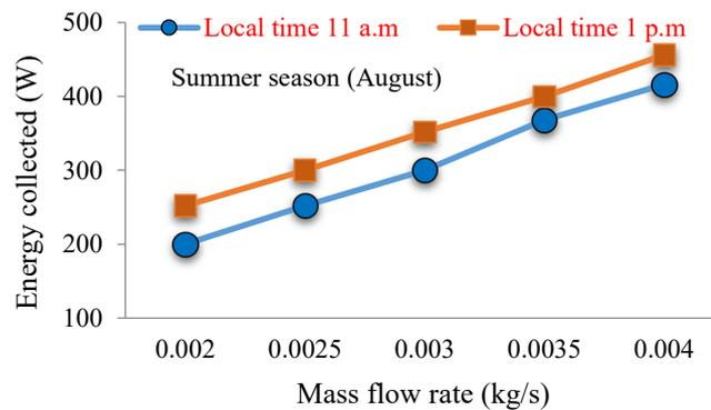
Figure 9. The variation of energy collected with mass flow rate of water
