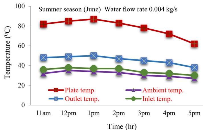
Figure 4. Variation of temperature during day time from 11 a.m. to 5 p.m.
