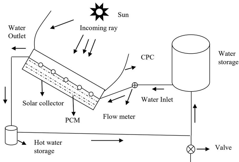
Figure 2. Schematic presentation of a thermal solar collector
