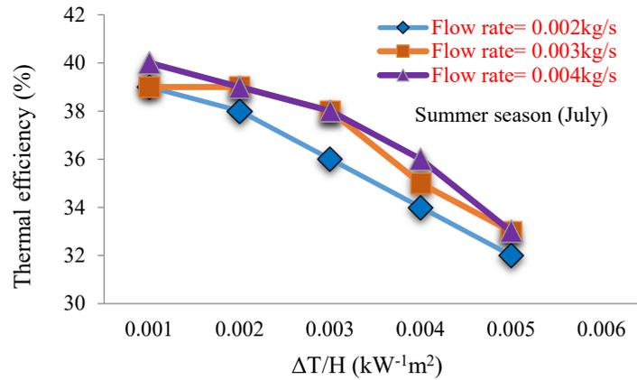
Figure 7. Thermal efficiency of thermal solar collector system for the corresponding  $\Delta T/H$  operating values
