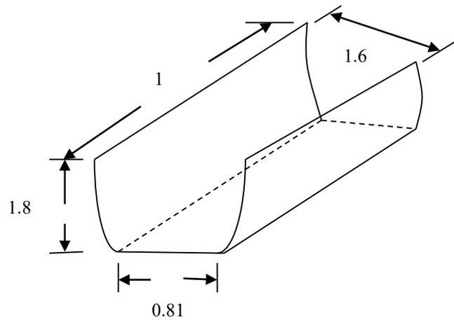
Figure 3. The geometry of a compound parabolic concentrator. (All dimensions are in meter)
