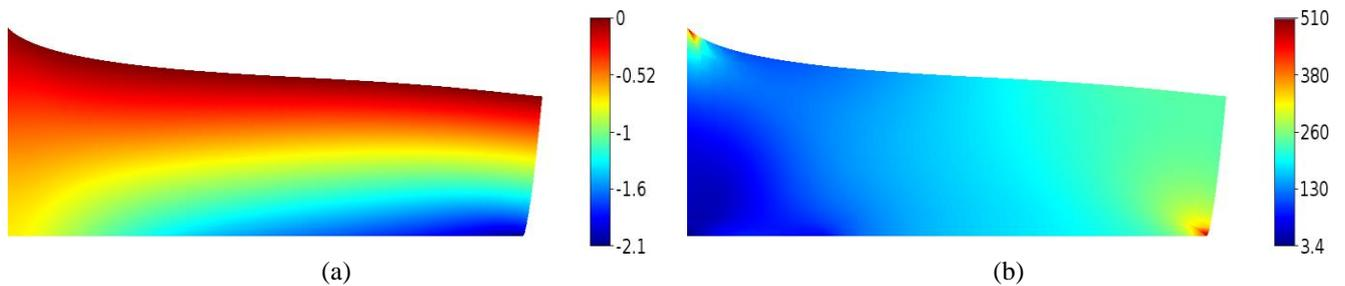
Figure 4. (a) Electric potential [V], (b) the Von Mises stress norm [Pa] at final time
