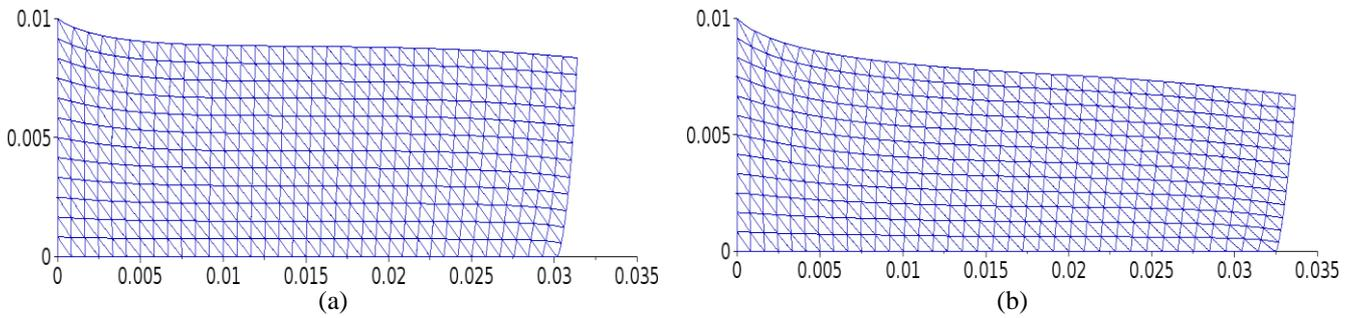
Figure 2. Amplified deformed mesh for (a) an insulated foundation, (b) a conductive foundation
