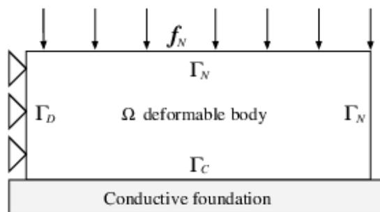
Figure 1. Contact problem with a conductive foundation
