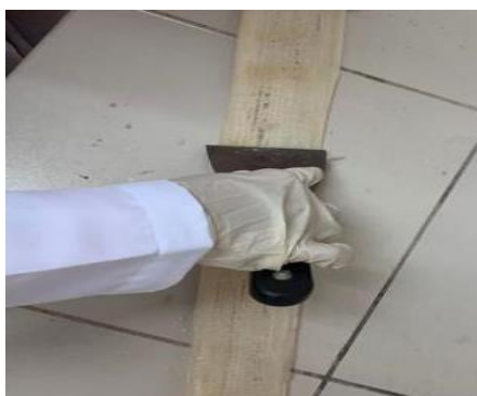
Figure 1. Scraping process of banana pseudo-stem fibres
