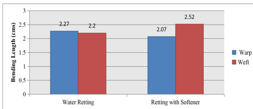
Figure 9. Bending length for stiffness test
