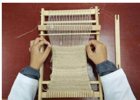
Figure 4. Weaving process using hand loom
